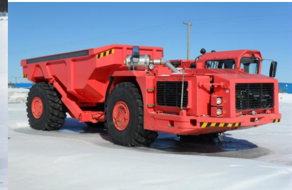
New 50t underground truck
