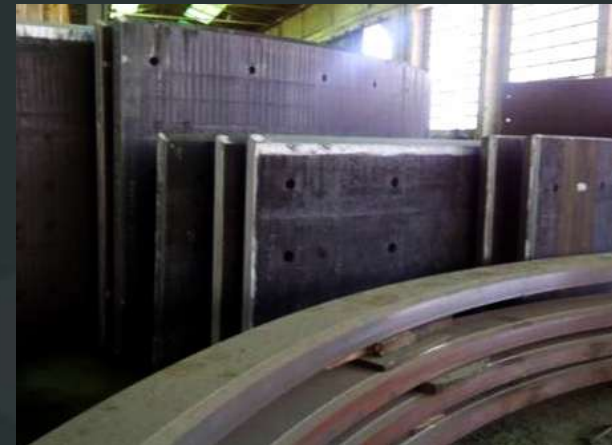
SHELL PLATE OF NEW SAG MILL
