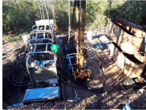
Portable diamond core rig for limited-access sites
