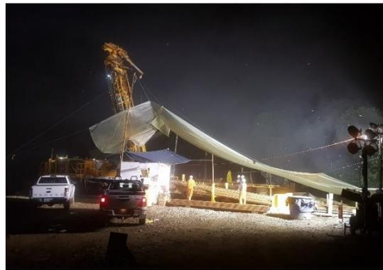
Track mounted rigs drill to 2800m at up to 90m per day
