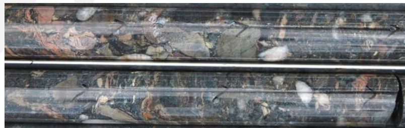
Tarkwaian conglomerate drill core from Anumso, Ghana
